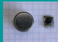
An iButton thermochron (left) and the circuit once removed for repackaging. Grid is 1 cm.
